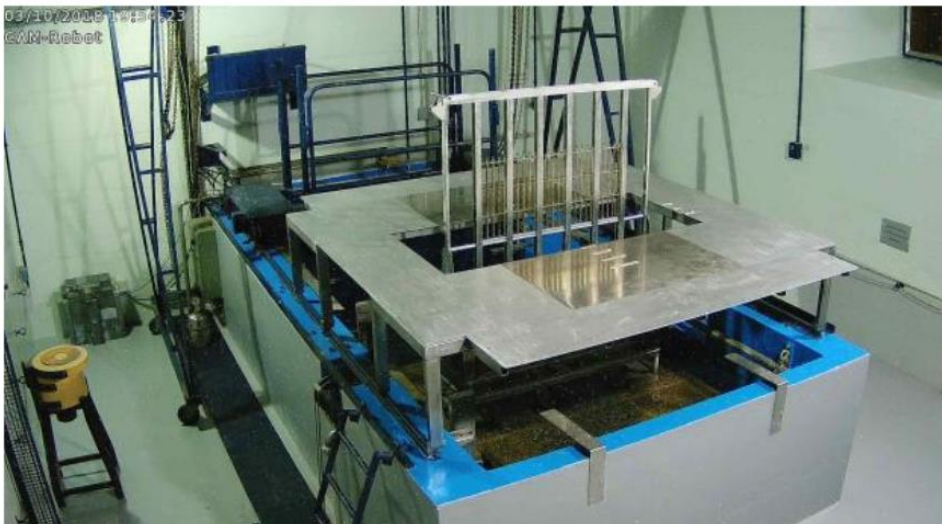
Figure 1: Irradiation cell with 60 Co sources rack and the platform for sample positioning.
